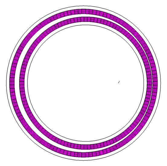
Solve the model and calculate the torque at (0,0) will give actual torque value 1.88858E+04 (lbf\*ft)
