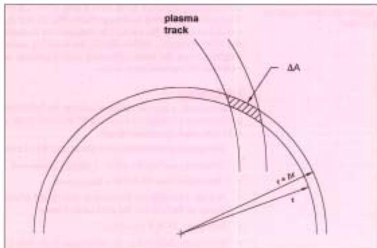
Figure 5 Principle of rotating magnet track design to generate a desired erosion profile. The relative plasma erosion from  $r$  to  $r + \Delta r$  is proportional to the area of interaction  $\Delta A$  relative to the total area of the band  $2rt$ . To make the erosion at  $r$  as small as possible, the plasma track should cross the band radially; for substantial erosion, the track should skirt tangentially along the band for a long distance.
