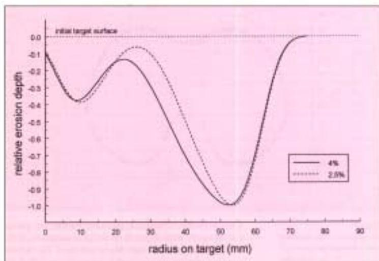
Figure 4 Two optimized erosion profiles designed for operation at a source-substrate distance of 3.5 mm. One profile is predicted to give  $\pm 4\%$  thickness uniformity, and the other  $\pm 2.5\%$ . The profile with the better uniformity has less inventory.
