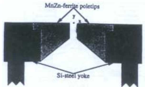
Figure 1: Partial geometry of a large-scale ring head used for BEM. Gap Length = 0.953 cm. Throat height = 2.337 cm. Turns = 200.
