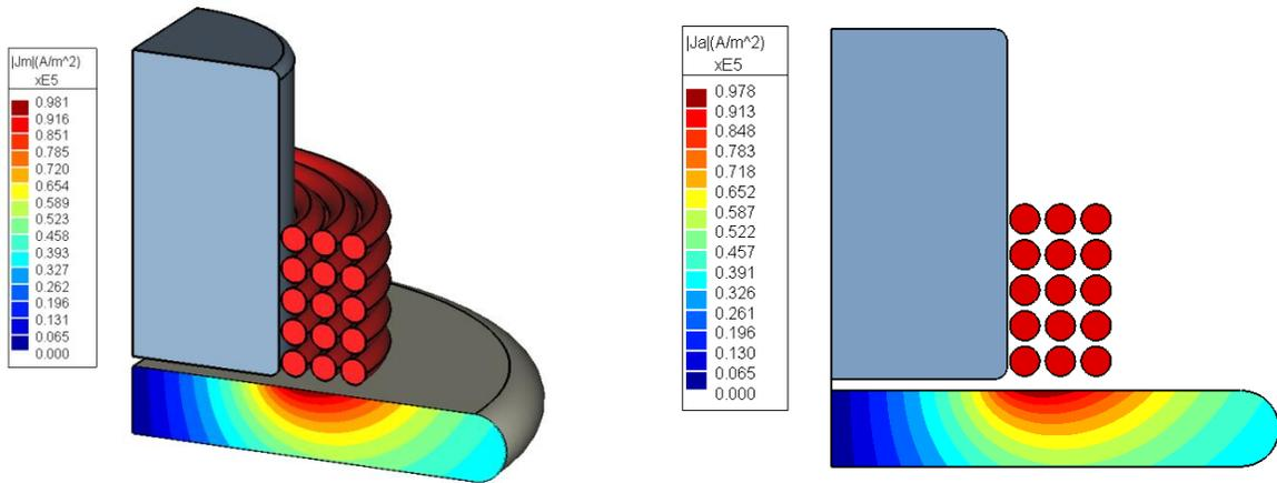
For models which are long in one dimension a **2D** approximation would be more appropriate. The **3D** and **2D** equivalent models for this situation are shown below.
