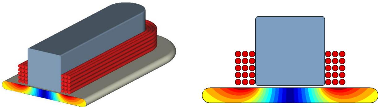
The coil examples we have shown have relatively few turns, and could be modeled directly in **3D** software, though simulation times would become significant if multiple solutions for different gaps were required (as would usually be the case). Typical sensors may have windings consisting of hundreds of turns, which would at best lead to extremely long solution times, or at worst might even exceed available computer capacity.
