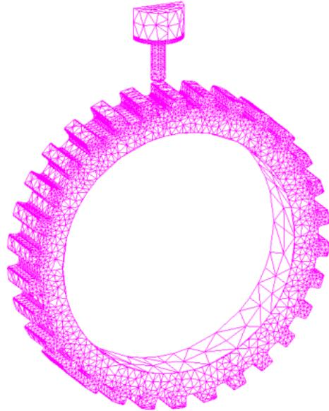
The next picture shows a reduced model where only one sixth of the gear is simulated. This model solves considerably faster, but still produces results which are within 5% of the full gear model.
