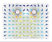
Rotational Symmetric model of Helmholtz coils showing vector potential contours and B field arrow plots
