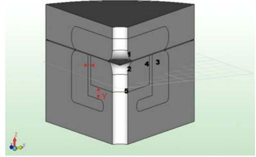
Figure 3. 3-D view of the electrode geometry used in computations. The parameters varied are ‘x’ & ‘y’ and stresses at locations 1-5 are examined.
