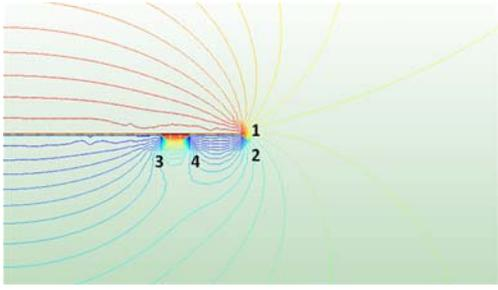
Figure 2. Electric field results produced by the BEM solver. Electrical stresses in V/m were determined at points 1, 2, 3 and 4.
