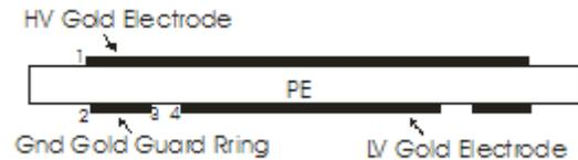
Figure 1. Simplified electrode geometry with polyethylene sandwiched between upper and lower gold electrodes.
