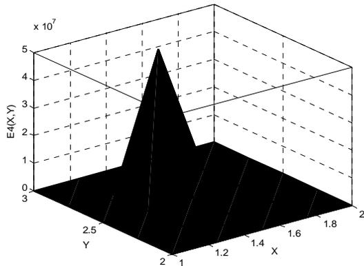
Figure 9. Electric field intensity (V/mm) plots for the point 4 for various values of the distance X and Y.
