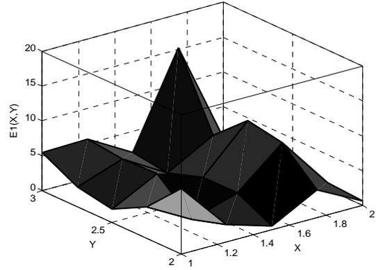
Figure 6. Electric field intensity plots (V/mm) for the point 1 for various values of the distance  $X$  and  $Y$ .
