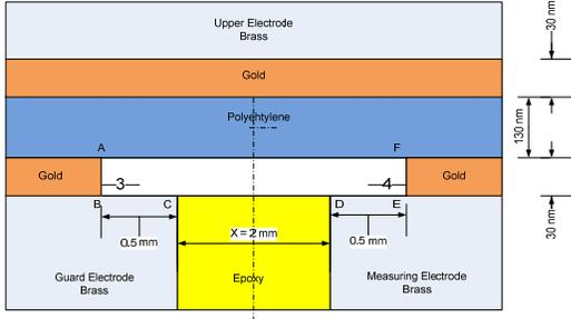
Figure 5. Expanded view (not to scale) of the electrode plane geometry showing the regions 3 and 4 and the relative dimensions of the various parts.
