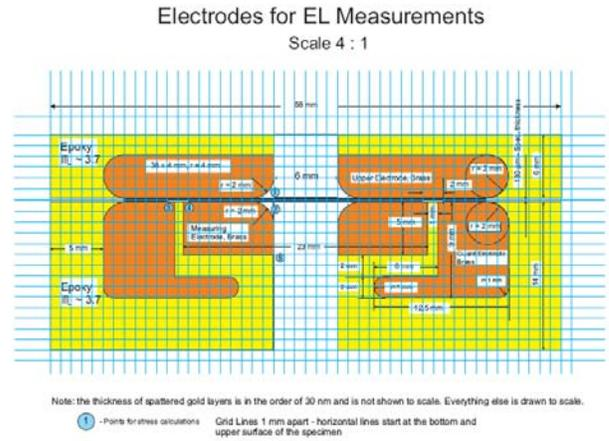
Figure 4. Electrode plane geometry with gold sputtered polyethylene sandwiched between upper and lower brass electrodes. Points 1, 2, 3, 4, and 5 were the locations used for the measurements of electrical stresses.
