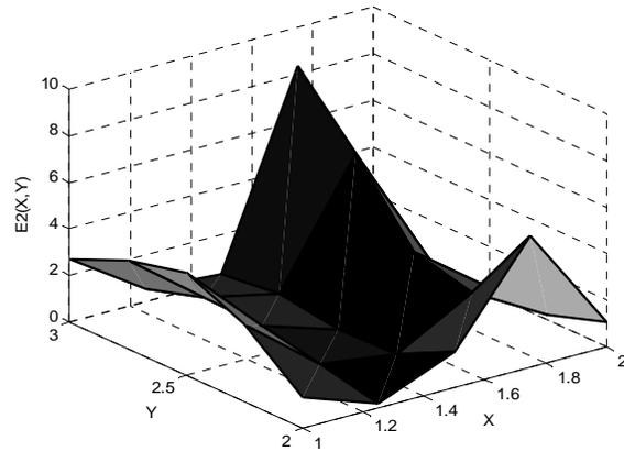
Figure 7. Electric field intensity (V/mm) plots for the point 2 for various values of the distance  $X$  and  $Y$ .
