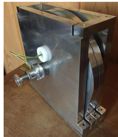
Fig. 9 Reluctance Motor completed in the machine work shop of the ETH in Zurich.
