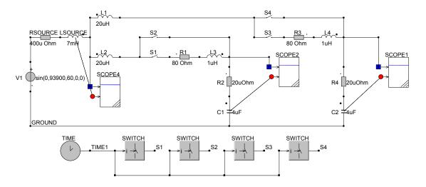
In this model diagram, inductors, capacitors, and resistors are clearly shown. Oscilloscope blocks are attached to the circuit to monitor voltages and currents. Switches are shown in the circuit and their associated control blocks shown below the schematic. Each switch block has its closing time programmed as a parameter for that block.
