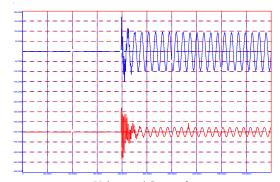
Voltage and Current for Energization of 2<sup>nd</sup> Bank at 5.5 Ohms
