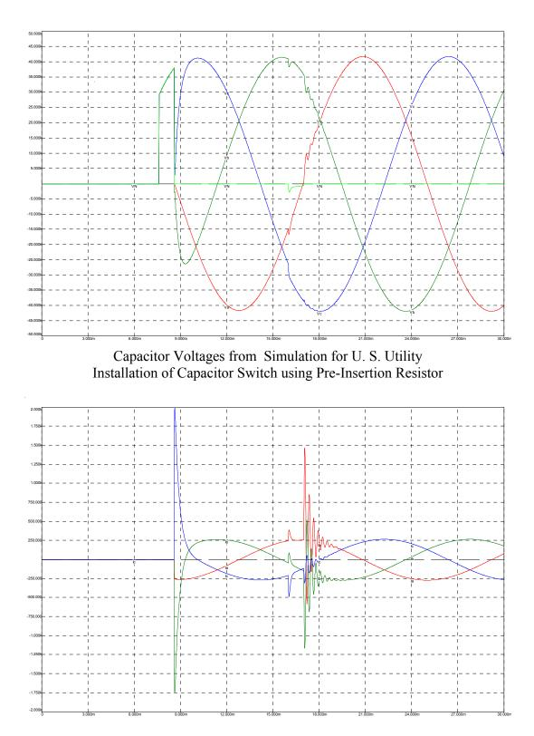
Capacitor Currents from Simulation for U. S. Utility Installation of Capacitor Switch using Pre-Insertion Resistor
