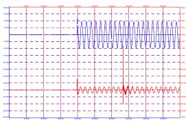
Voltage and Current for Energization of 2nd Bank at 81 Ohms
