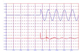
Voltage and Current for Energization of 2<sup>nd</sup> Bank at 80 Ohms
