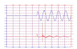
Voltage and Current for Energization of 2<sup>nd</sup> Bank at 150 Ohms
