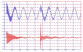
Voltages and Current for Energization of 1<sup>st</sup> Bank
