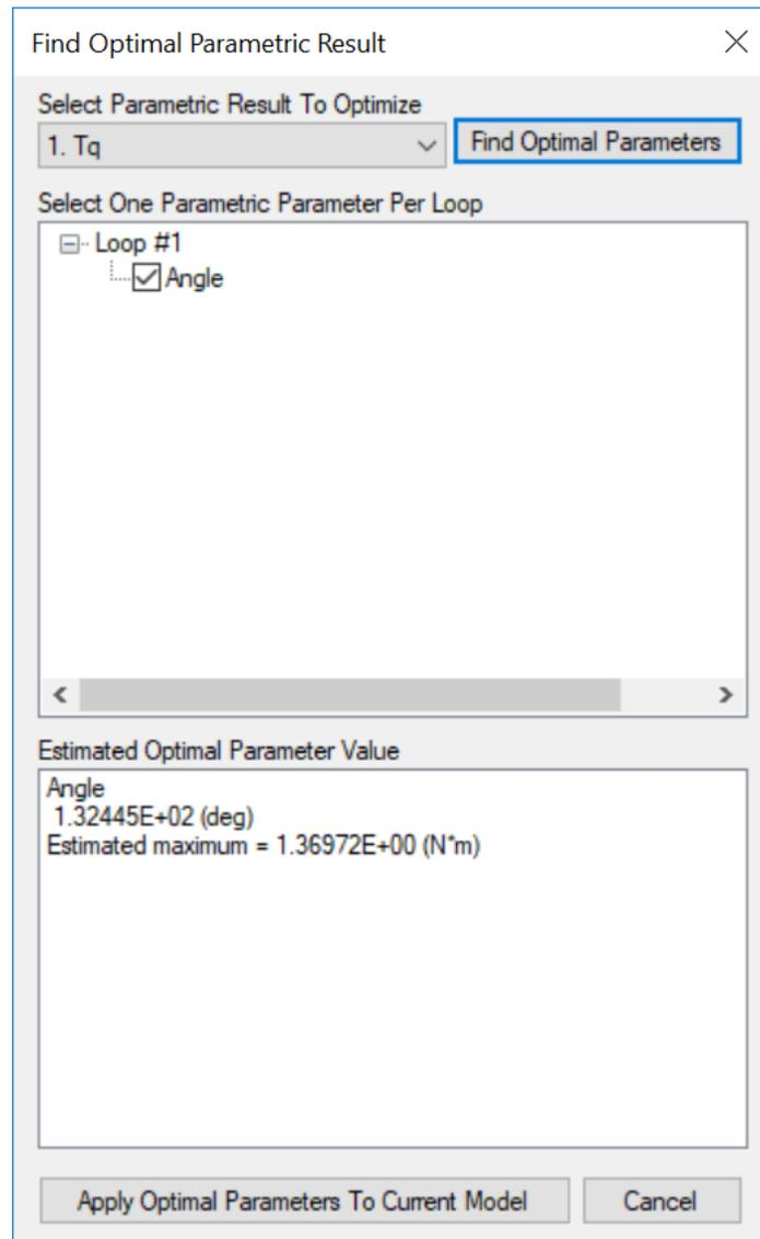
IMPORTANT: If you have more than one parametric variable defined in a loop, it is important to define all the parametric variables to be dependent to a single parametric variable in the loop. **The optimization algorithm can only optimize one parametric variable per loop.** If a parametric variable cannot be made dependent on another parametric variable in the same loop, consider moving the parametric variable to a new loop. Failure to follow this rule would produce erroneous results.
