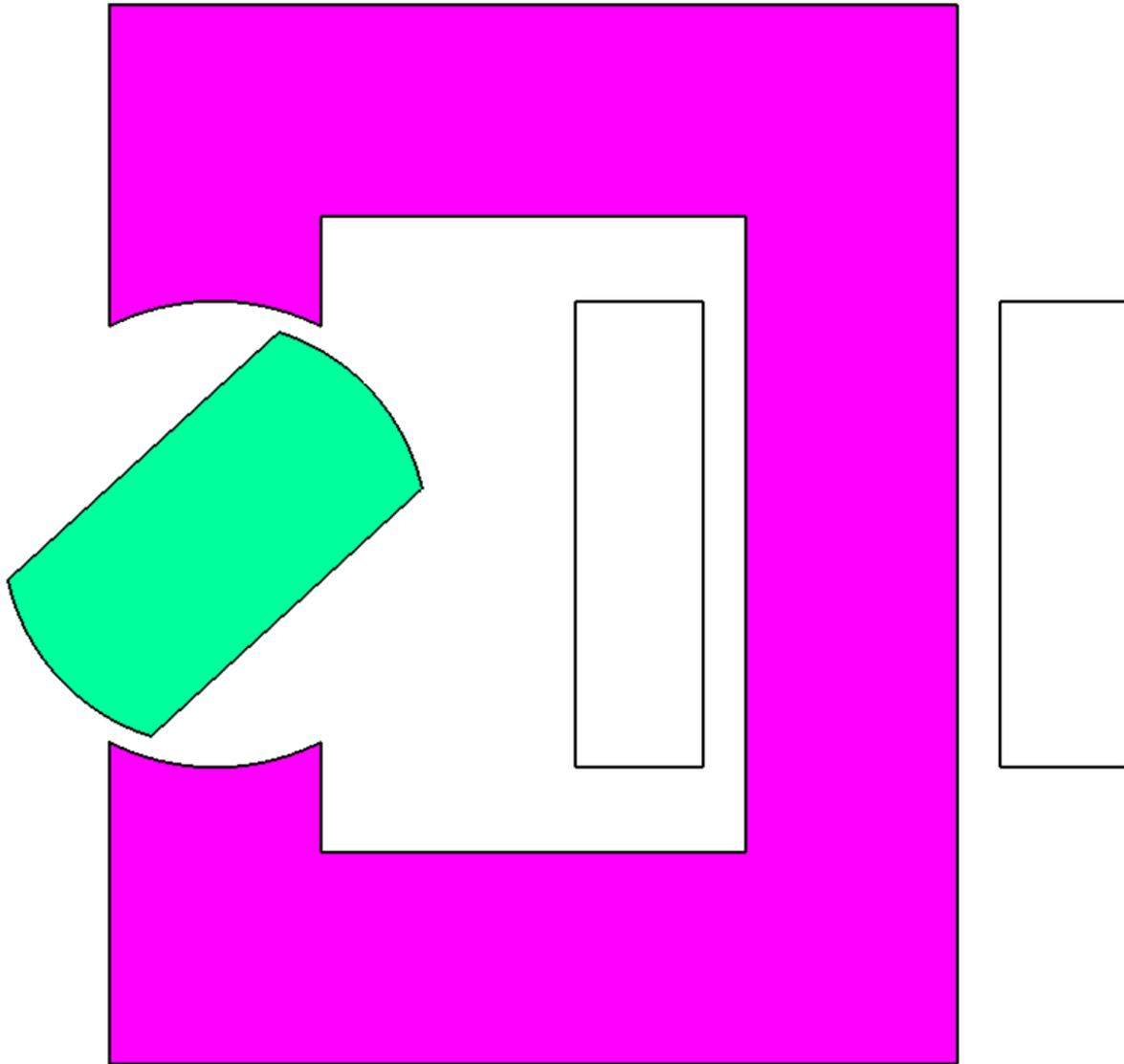
Solving this model and calculating the torque of the permanent magnet at location (10, 50) will yield actual torque value 1.37 Nm.
