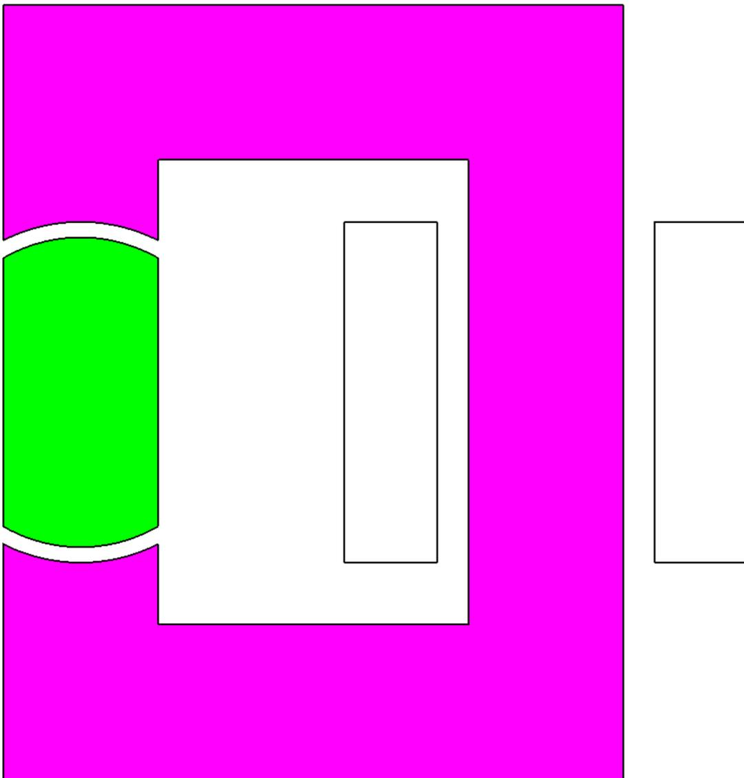
A 100 steps parametric run is setup to rotate the permanent magnet and torque is calculated on the magnet for each step.
