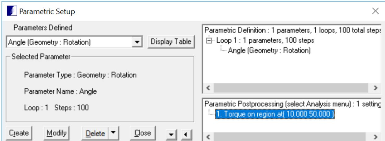
The permanent magnet is rotated from 0 to 180 degrees in 100 steps.
