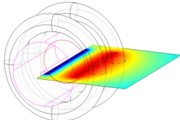
The contour plot above shows voltage on a plane slicing through the two cylinders. The plot shows that inside the cylinders the voltage is quite uniform along the direction of the axis. As expected there are fringing effects at the ends of the cylinders.
