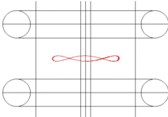
The fringing effects of the fields in the chosen geometry and release position for the electron are hence seen to act as a trap serving to confine the electron motion along the axis to a 4.1 MHz oscillation.
