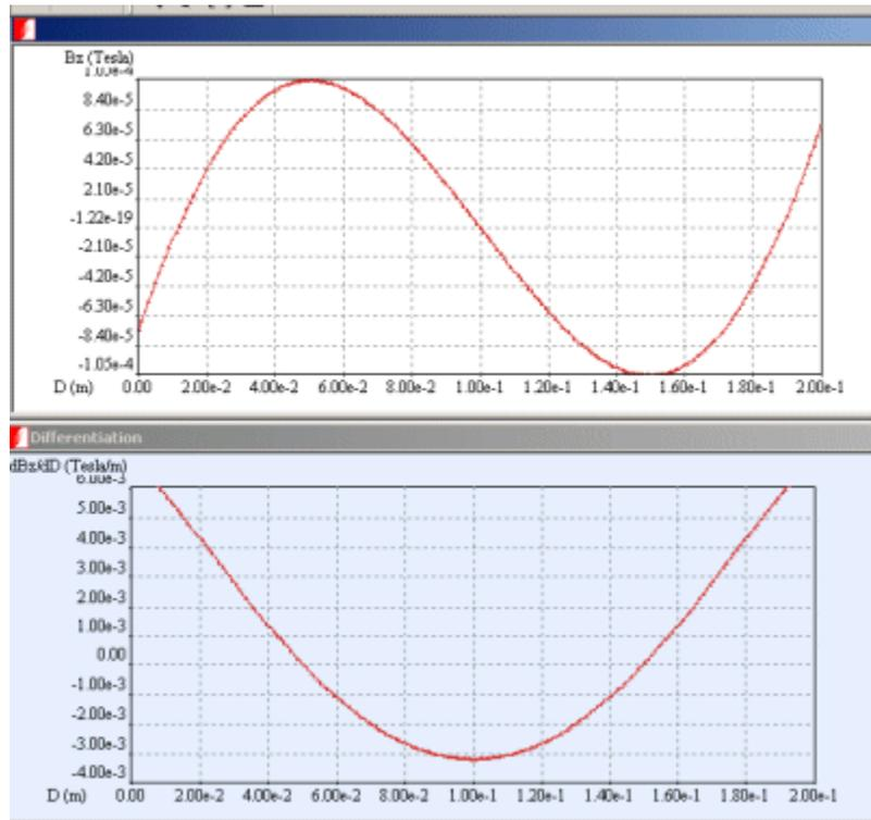
As seen above, the "spring constant" due to B decreases as the particle moves further away from the center. However, the "spring constant" for E increases and the two effects will cancel out to some extent. To the left is a screen shot of an orbit resulting from releasing the electron from rest at a radius of 0.12 m at a height of 0.01 m above the center. The observed frequency here is 4.10 MHz.
