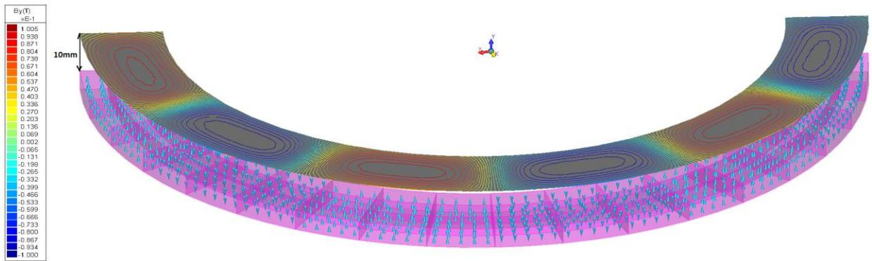
Fig.6: Magnetic charger deleted. Contours of the Y component of magnetic flux density vector B on a surface 10mm above the magnetized semicircular ring.
