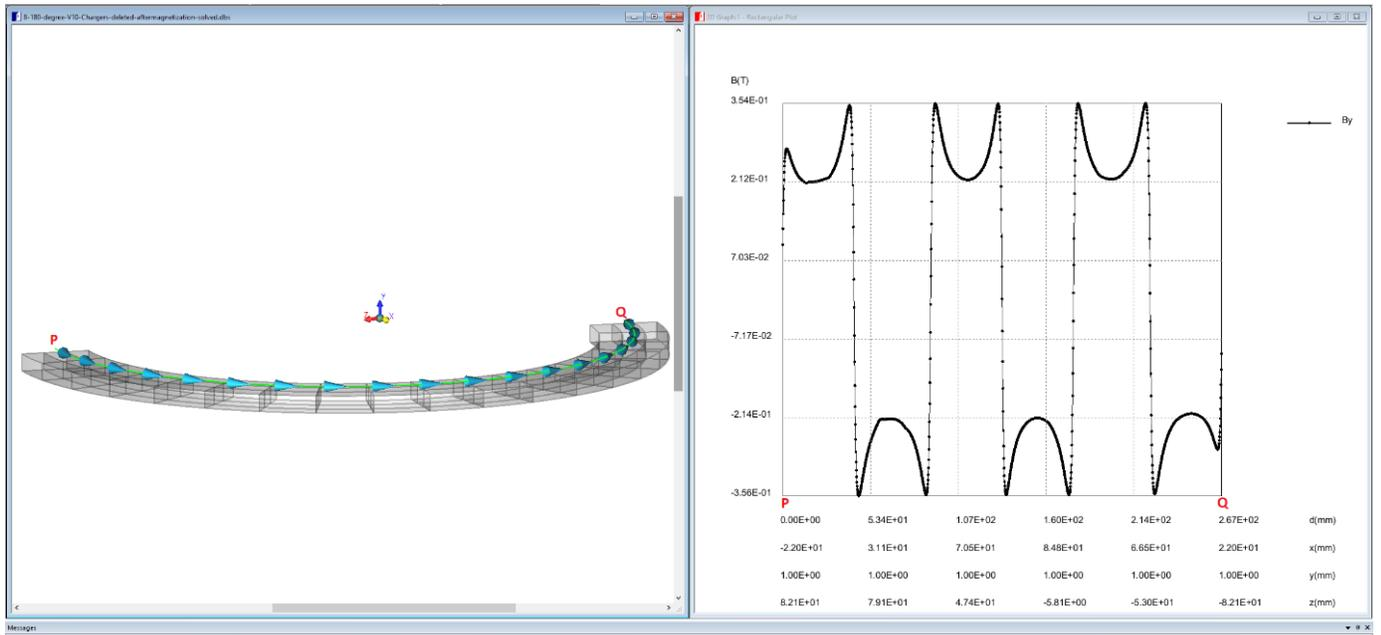
Fig. 7: Variation the Y component of magnetic flux density B along a semicircular arc 1mm above the magnetized ring.
