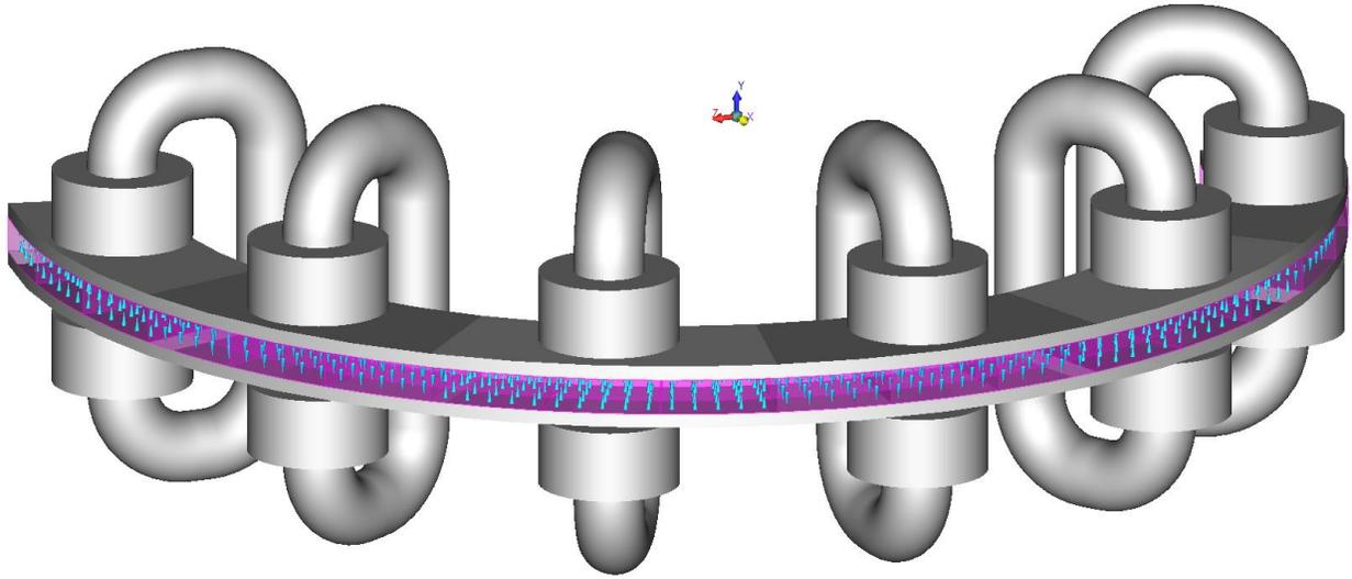
Fig. 5: Semicircular ring after magnetized.
