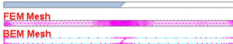
The model consists of a 1 m thick x 20 m long dielectric with relative permittivity=4 and conductivity=0. On top of the dielectric is a 40 m long 1 V electrode and underneath is a 40 m long 0 V electrode. To force the interior to become semi-infinite at the ends a linear voltage condition of 0-1 V is applied to the two 1 m tall ends.
