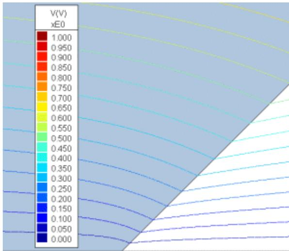
One of the most common questions in Electromagnetic simulation is "what/where is the maximum field?". When a junction is present the question becomes tricky. In the sample case to the left the "triple junction" is a dielectric (left), air (right) and an electrode (bottom). Although the voltage looks well behaved, this junction is mathematically a singularity.
