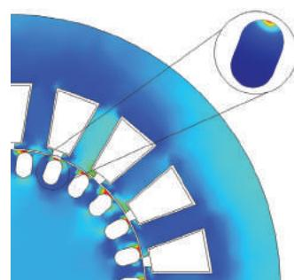
Field magnitude plot in the rotor and stator of an induction motor; current density induced in one rotor bar (inset)
