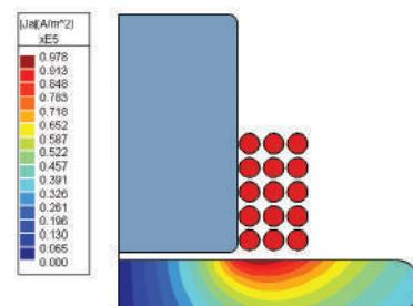
Rotational Symmetric model of an eddy current sensor showing current density contours induced in target
