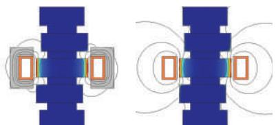
One of the major challenges in the induction hardening of steel camshafts relates to the avoidance of undesirable heating in adjacent areas that have previously been hardened (temper back effect).
