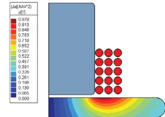
Rotational Symmetric model of an eddy current sensor showing current density contours induced in target
