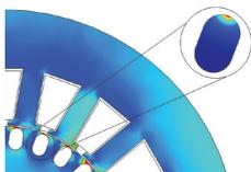
Field magnitude plot in the rotor and stator of an induction motor; current density induced in one rotor bar (inset)
