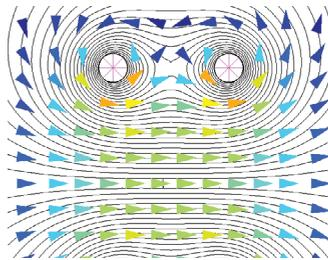
Rotational Symmetric model of Helmholtz coils showing vector potential contours and B field arrow plots
