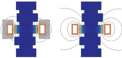
One of the major challenges in the induction hardening of steel camshafts relates to the avoidance of undesirable heating in adjacent areas that have previously been hardened (temper back effect).
