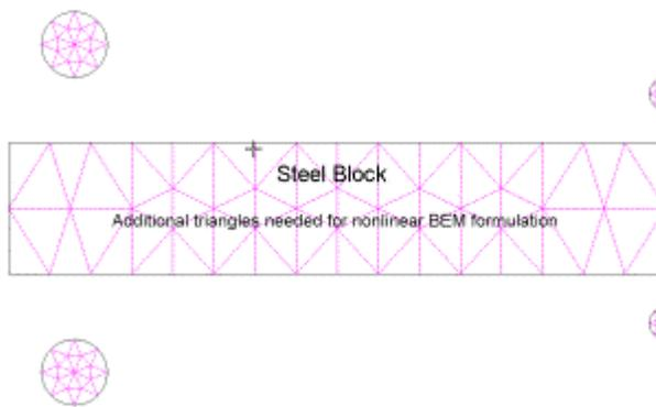
Figure 4: Additional Unknowns for Nonlinear BEM
