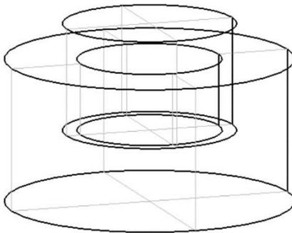
These kinds of intersections can be automatically detected by using the Geometry > Detect > Intersecting Volumes command. This function cycles through all the volumes in the model and tests for intersections with other volumes. Volumes that are found to intersect are highlighted as they are found for the user to review as below:
