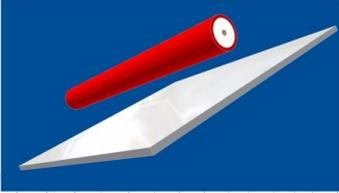
In Fig.1, a high voltage cable is shown, one cable diameter (5.2mm) from a grounded plate. The cable construction is 7/0.3mm core and the insulation is polyethylene with a PVC sheath. The cable is rated at 25kV and in this case, the potential difference is 20kV.
