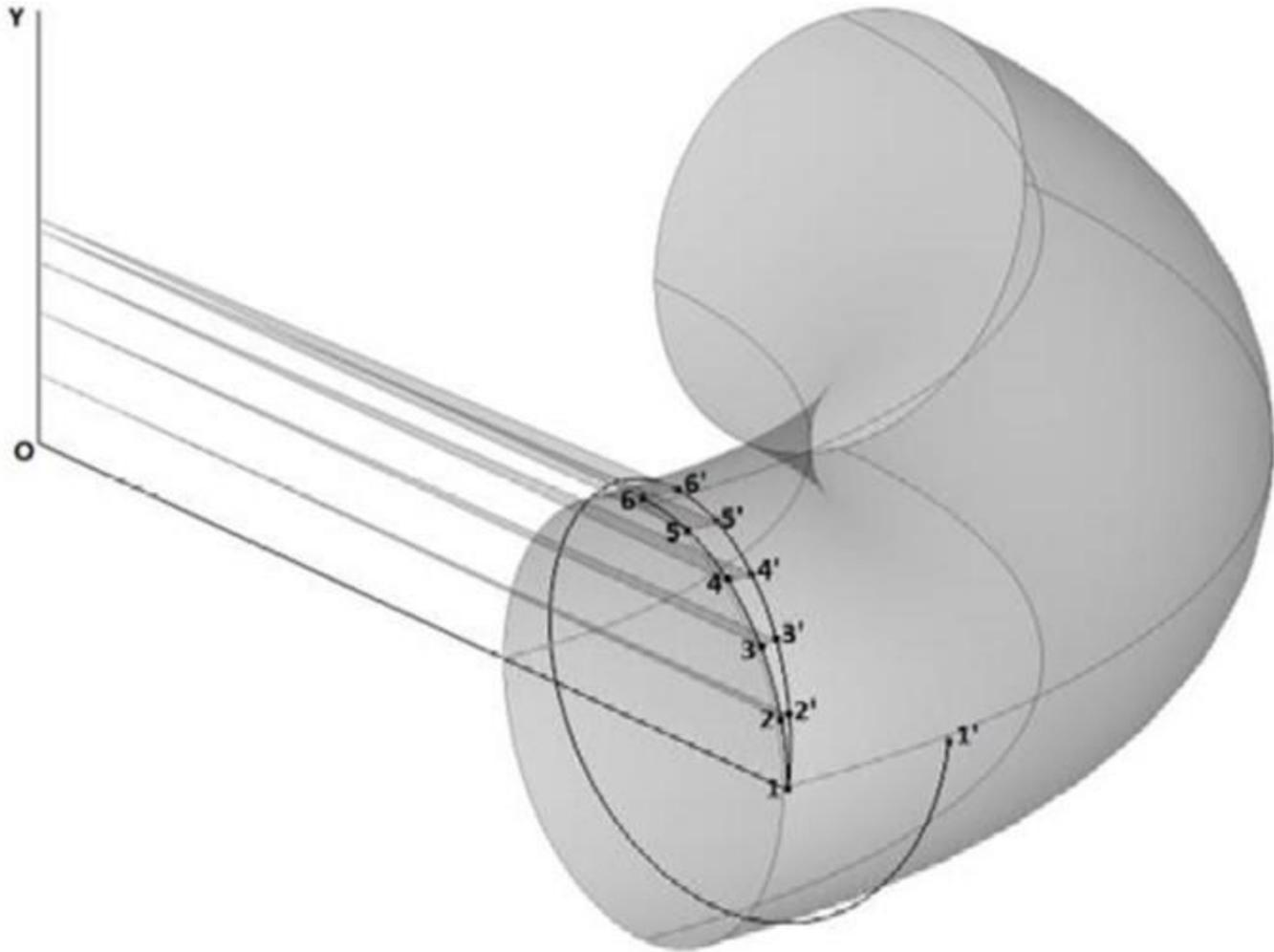
**Fig. 1: Winding a point on a toroid**
