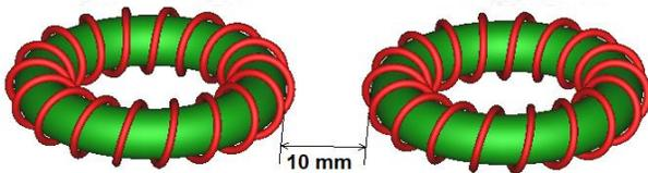
Fig. 4: Two identical coils of specs given in Fig. 2 are placed side by side.
