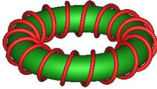
Fig. 2: Mean Radius of Toroid =13mm, Radius of Toroid cross section = 3mm, Wire Radius = 0.5mm, Number of Turns = N = 18, Gap between Wire and Toroid = 0.1mm, Relative permeability of Toroid –  $\mu_r$
