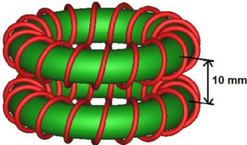
Fig. 3: Two identical coils of specs given in Fig. 2 are placed axially one above the other.
